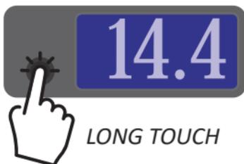
To switch between display modes and edit parameters, use QUICK TOUCH. To enter programming mode, use the LONG TOUCH. To save changes and exit programming mode, press LONG.
